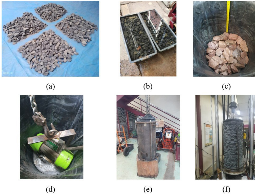
Figure 6. (a) Sample Quartering; (b) Submersion; (c) Mold filling; (d) Sample densification; (e) Top-cap placement; (f) Vacuum application.
